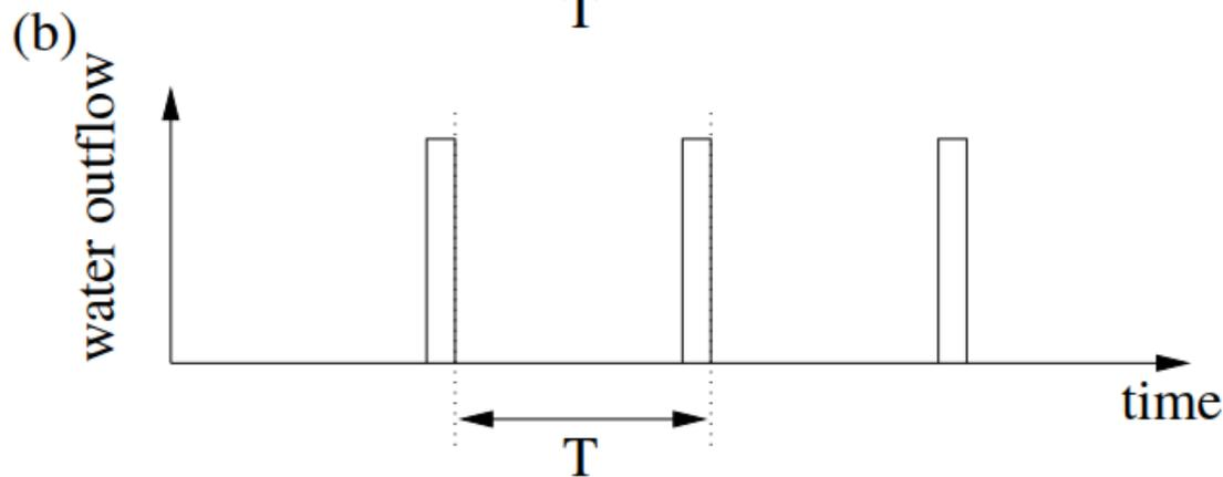
*Time course of the mechanical integrate-and-fire (accumulate-and-fire) oscillator.*
