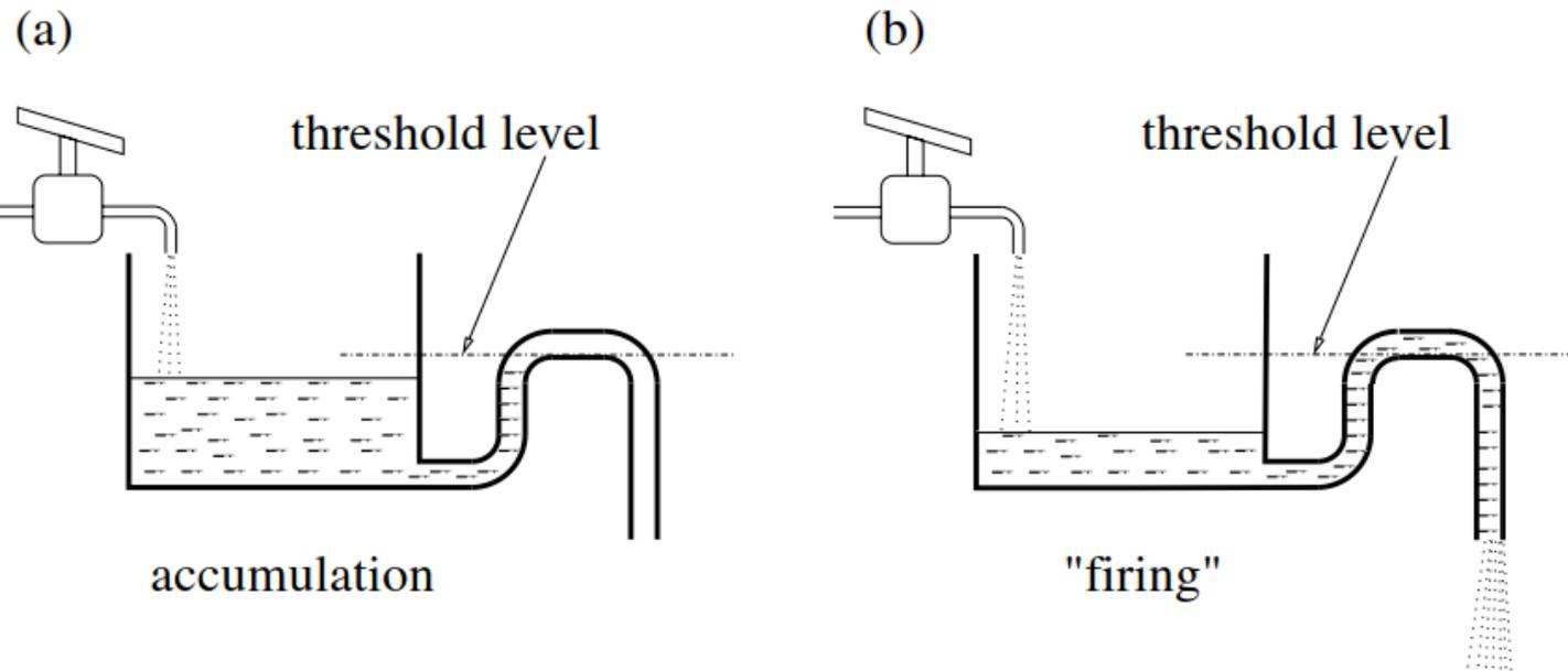
The energy of the pump that provides a constant water supply is transformed into oscillations of the water level in the vessel.
